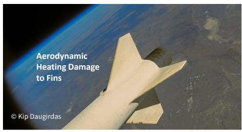
Surface Damage to Rocket from Mach 4 Aerodynamic Heating and Erosion from High Dynamic Pressure
